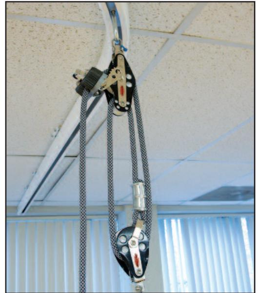
▲ This simple pulley system provides a 3/1 mechanical advantage for quick and easy adjustment. The unique "cam-cleat" allows for a secure hold but can be released and adjusted when needed with a simple flick of the wrist. The system is extremely lightweight, which allows for rapid and dynamic changes in direction.
