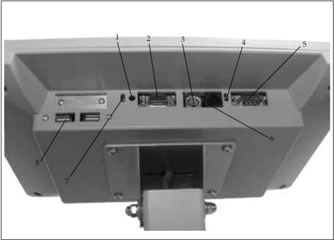
Figure 5.7 The printer power cable should be plugged into the AC receptacle on the rear base of the display support post. The printer USB cable should be plugged into the USB port on the back of the display.
