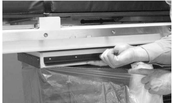
Figure 9. Lift the lower section of the strip on each side of the table, slide the plastic skirt underneath and lower the strip to hold the skirt in place.
